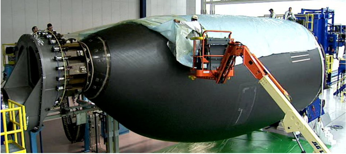
Figure 3: An airplane fuselage is manufactured with prepreg carbon fiber. Here, it is being sealed in a vacuum bag for a debulk or the final cure [6].
